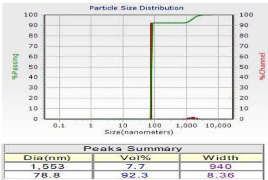
**Fig. 5. Dynamic Light Scattering of Chitosan-Silver Nanocomposites.**
