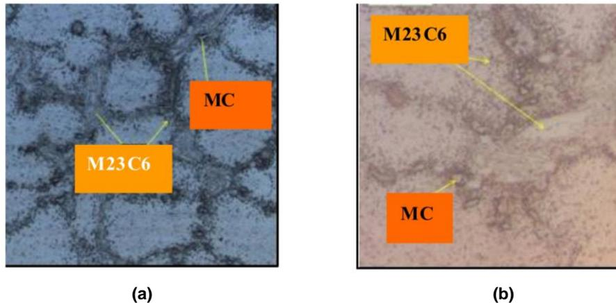
**Figure 3. Microstructures of two aged samples (a) before reaching the maximum hardness value and (b) after the maximum.**
