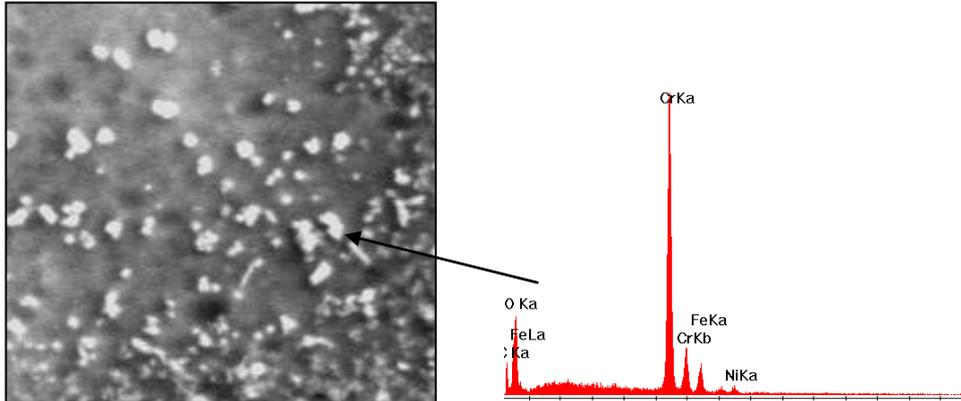
**Figure 5. Secondary precipitation of carbides in an over-aged sample.**
