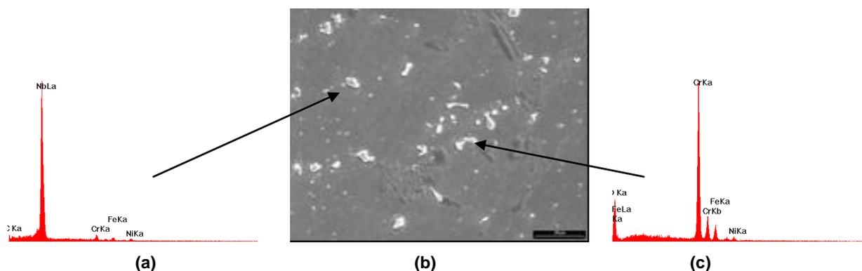
Figure 2. As cast microstructure observed by scanning electron microscopy (SEM) and EDAX spectra, corresponding to two types of carbides.
