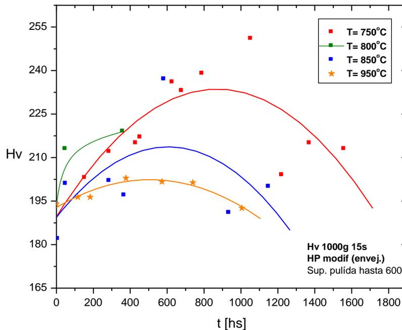
**Figure 4. Vickers hardness for four aging temperatures and different times.**
