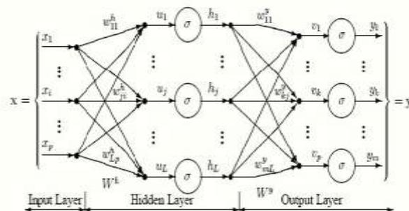
Figure 1 Multilayer Perceptron Neural Network Structure
