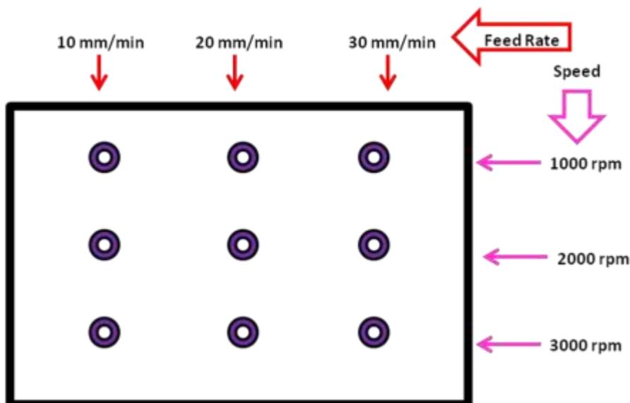
**Fig 1: Test specimens and drilling parameters for Carbon-Carbon composites**
