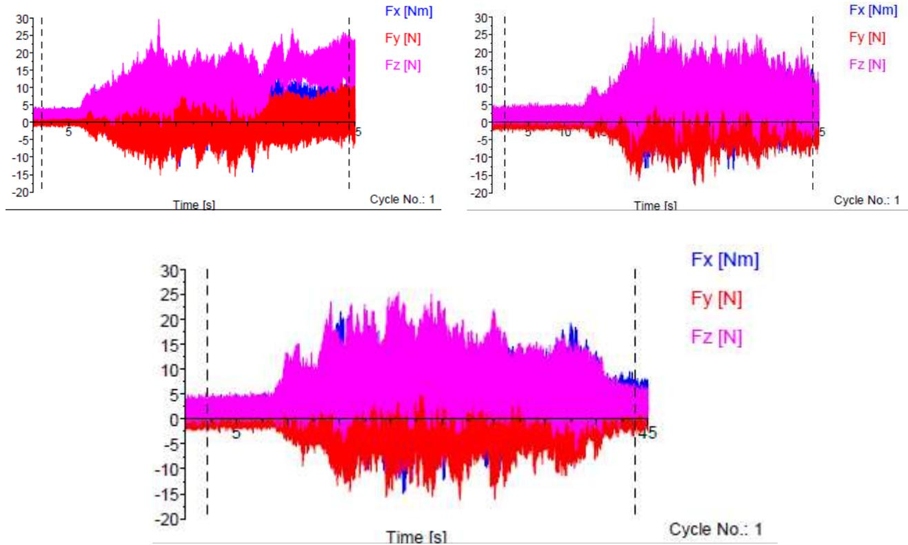
**Fig 2: Torque and thrust force Vs time of drilling for (a) 1000 rpm (b) 2000 rpm and (c) 3000 rpm @ 10 mm/min**
