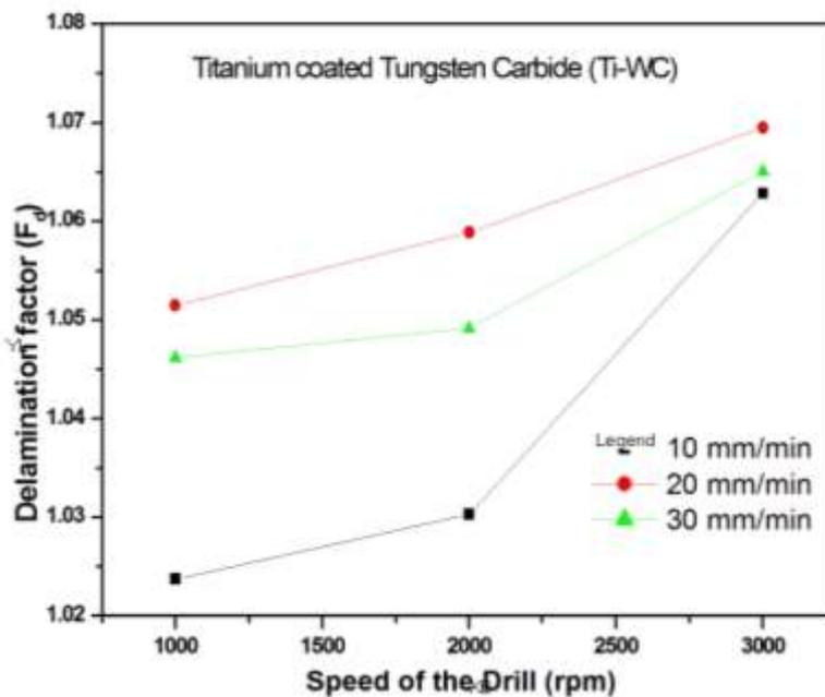
**Fig 5: Delamination factor ( $F_d$ ) for Ti-WC drill for various feed rate and drill speeds.**
