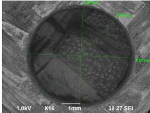
**Fig 4: Microscopic picture on the surface of the carbon-carbon composites with a drill speed of 3000 rpm at the feed rate of 10 mm/min.**
