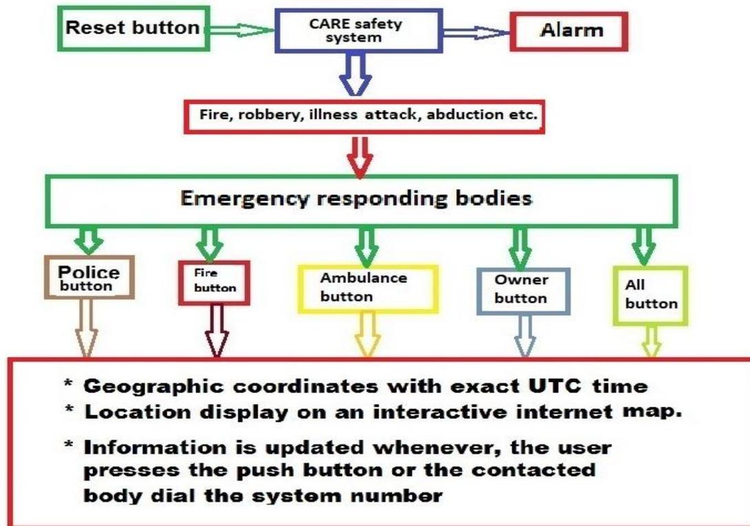
Figure 7, A flow chart showing the system functions sequence.
