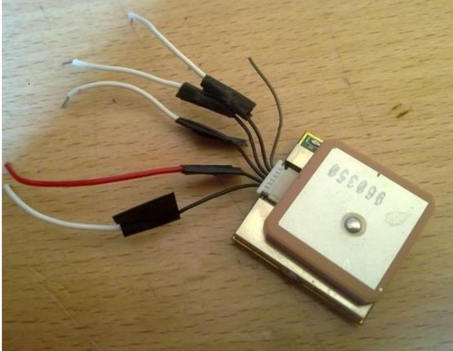
**Figure 4, The GPS unit of the CARE system.**
