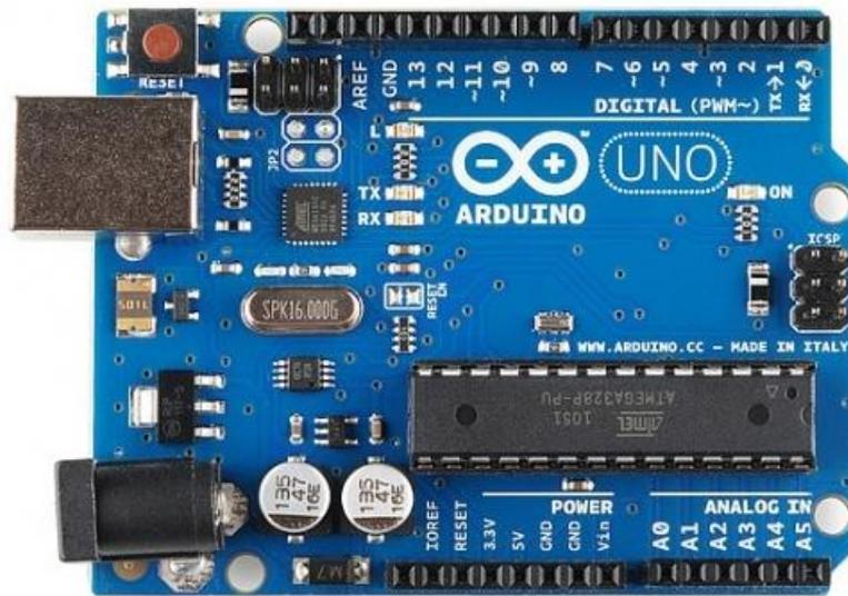
Figure 2, ARDUINO UNO unit of the CARE system
