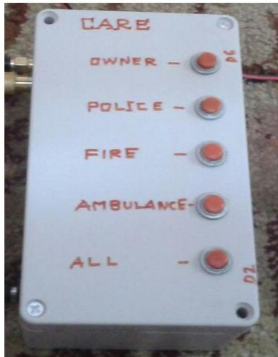
**Figure 6, The assembled CARE system with the programmed buttons**
