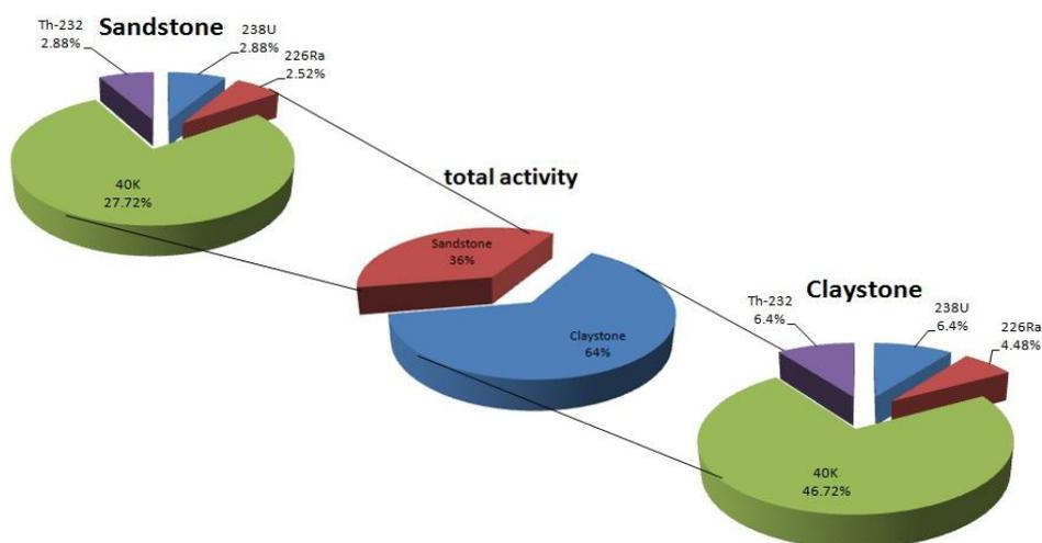
Fig.3: The distribution of natural radioactivity in the rock samples of Al-Obour city.
